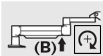
Figure 4-5. With Arm Horizontal, Tighten Set Screw (B)
