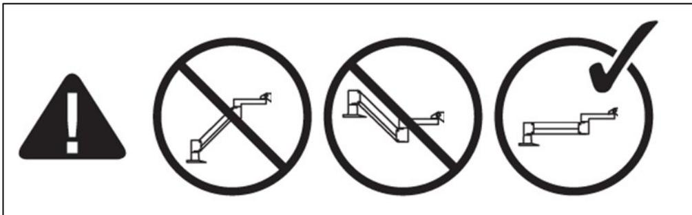
*Figure 4-2. Position the Arm Parallel to the Floor*
