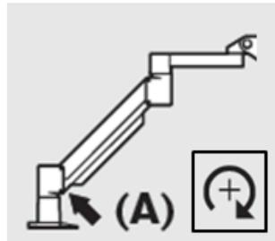
Figure 4-4. With Arm Raised, Tighten Set Screw (A)
