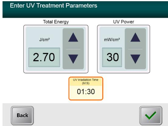
Figure 3-8. Pulsed UV Treatment Parameters Screen
