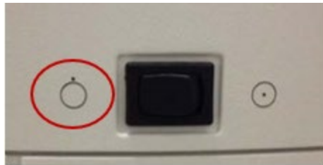
Figure 3-29. Power Off Position
