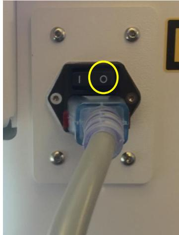
**Figura 3-50. Posición Apagar (Power Off)**
