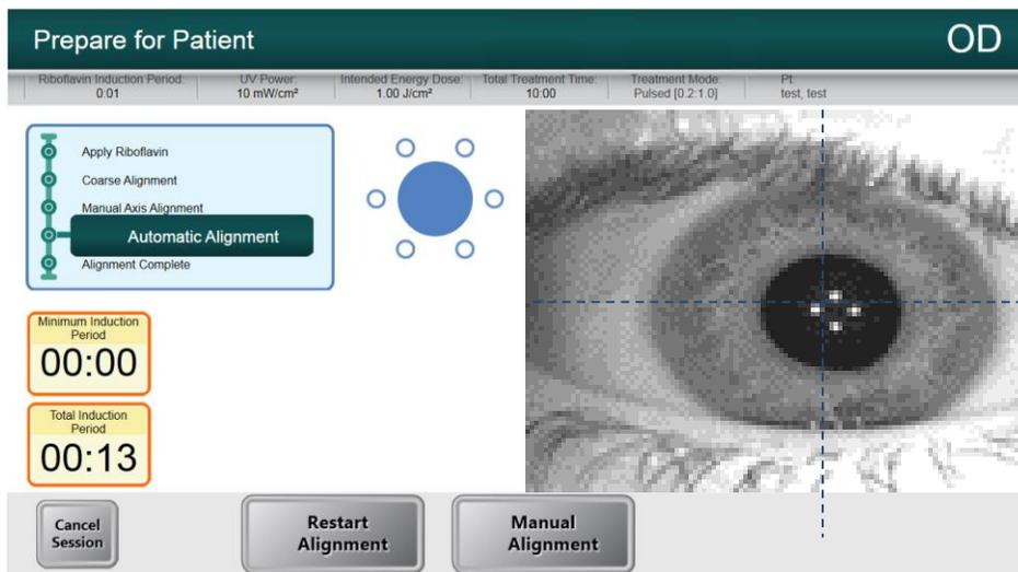
Figure 4-19 Re-start Auto Alignment or Manual Alignment Option
