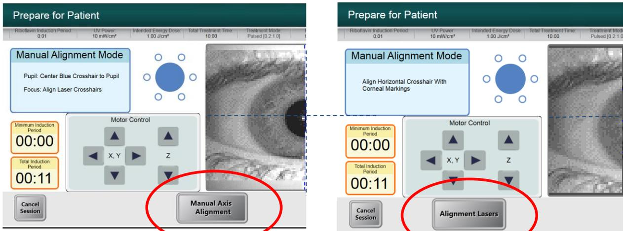
Figure 4-20 Toggling between Manual Axis Alignment & Alignment lasers
