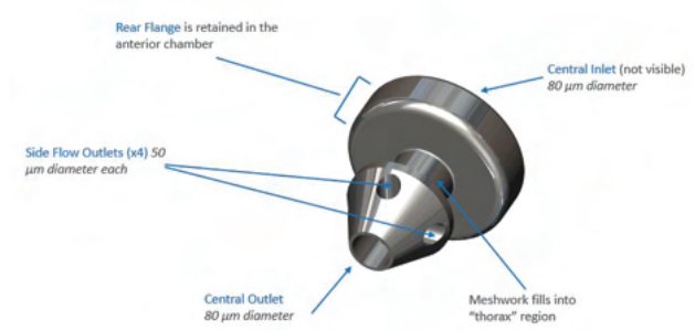
Figure 2. iStent infinite Stent (Model G2-W Stent)
