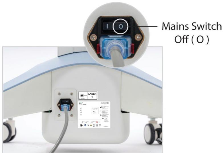
**Figure 34. Mains Power Switch in Off Position**
