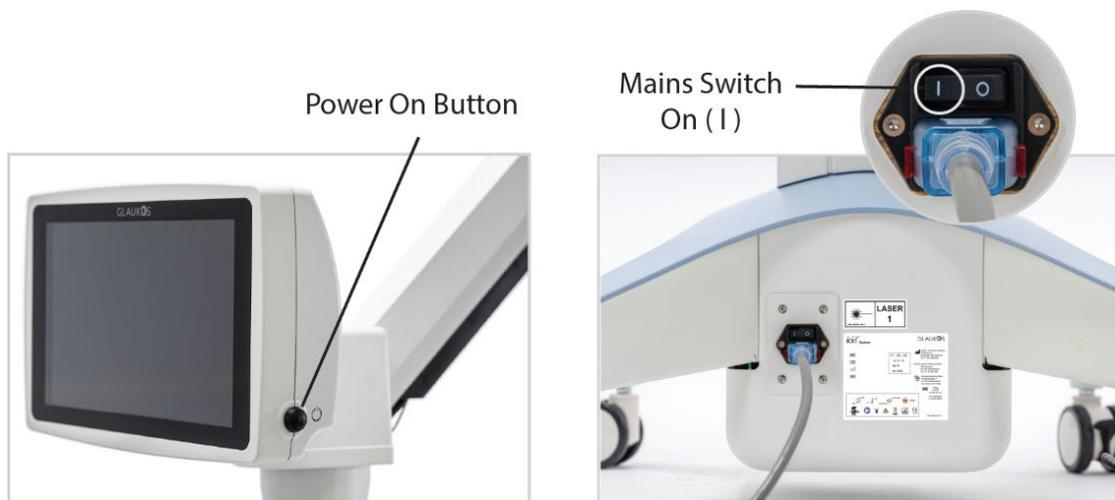
Figure 7. Power-on Button (left) and Mains Power Switch (right)
