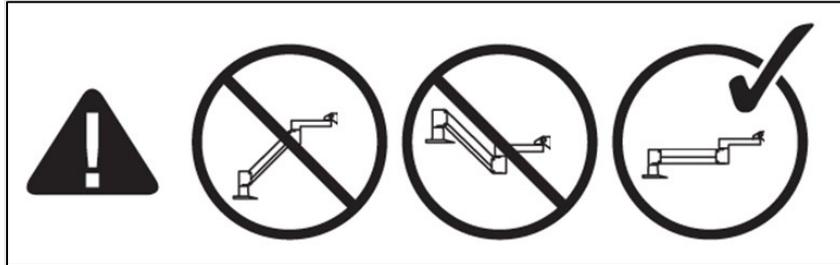
**Figure 40. Position the Arm Parallel to the Floor**
