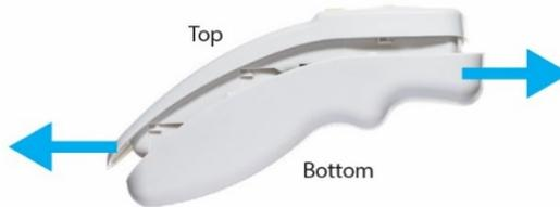
**Figure 37. Access Battery Compartment**
